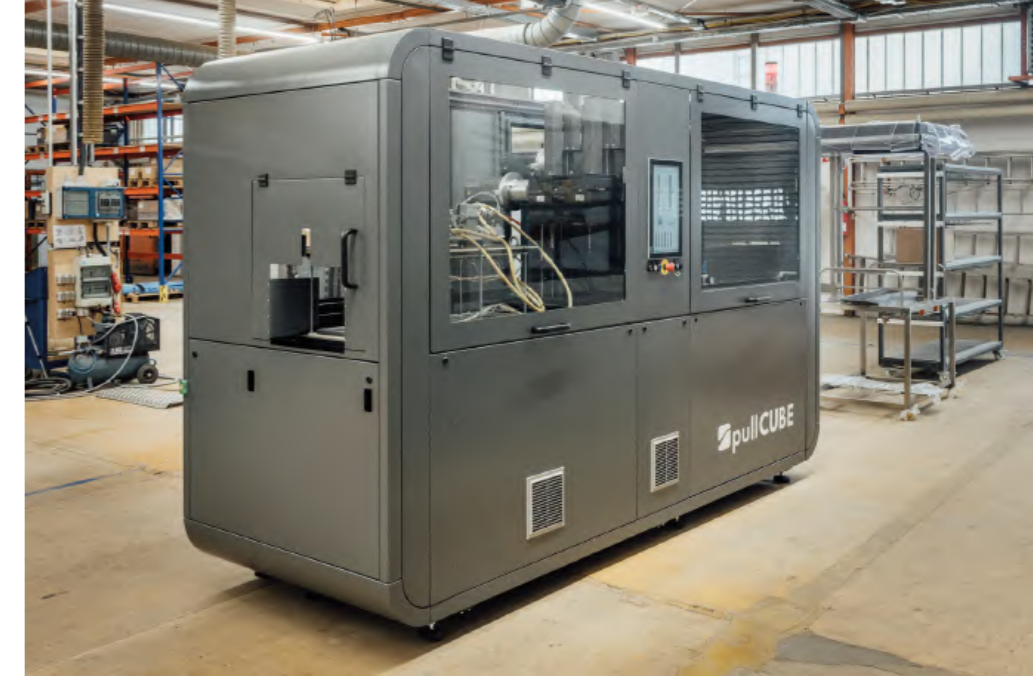
At 3.5 meters, the pullCUBE is the shortest pultrusion machine in the world
